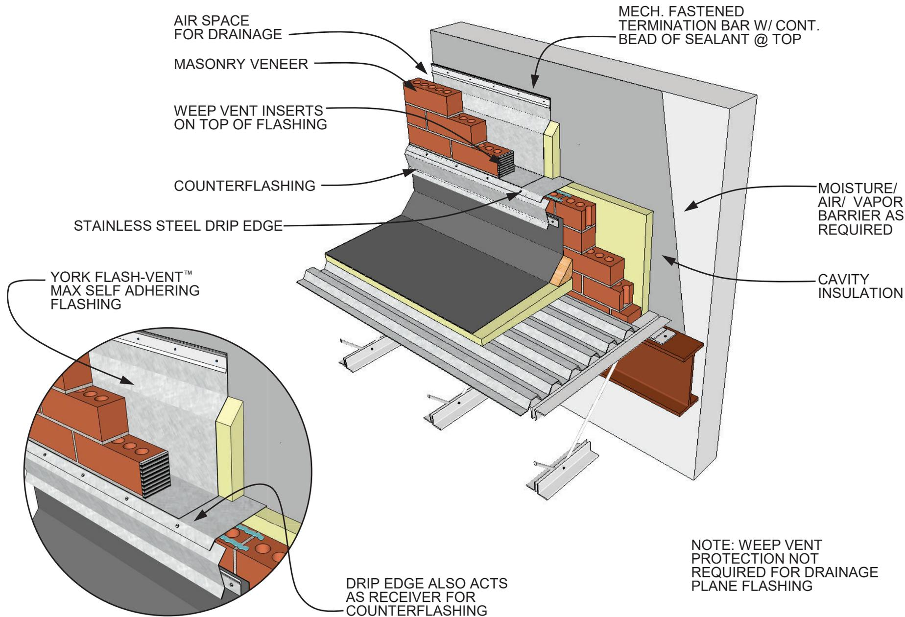
HIGH WALL/LOW ROOF DETAIL YORK FLASH-VENT™ MAX SELF ADHERING FLASHING
