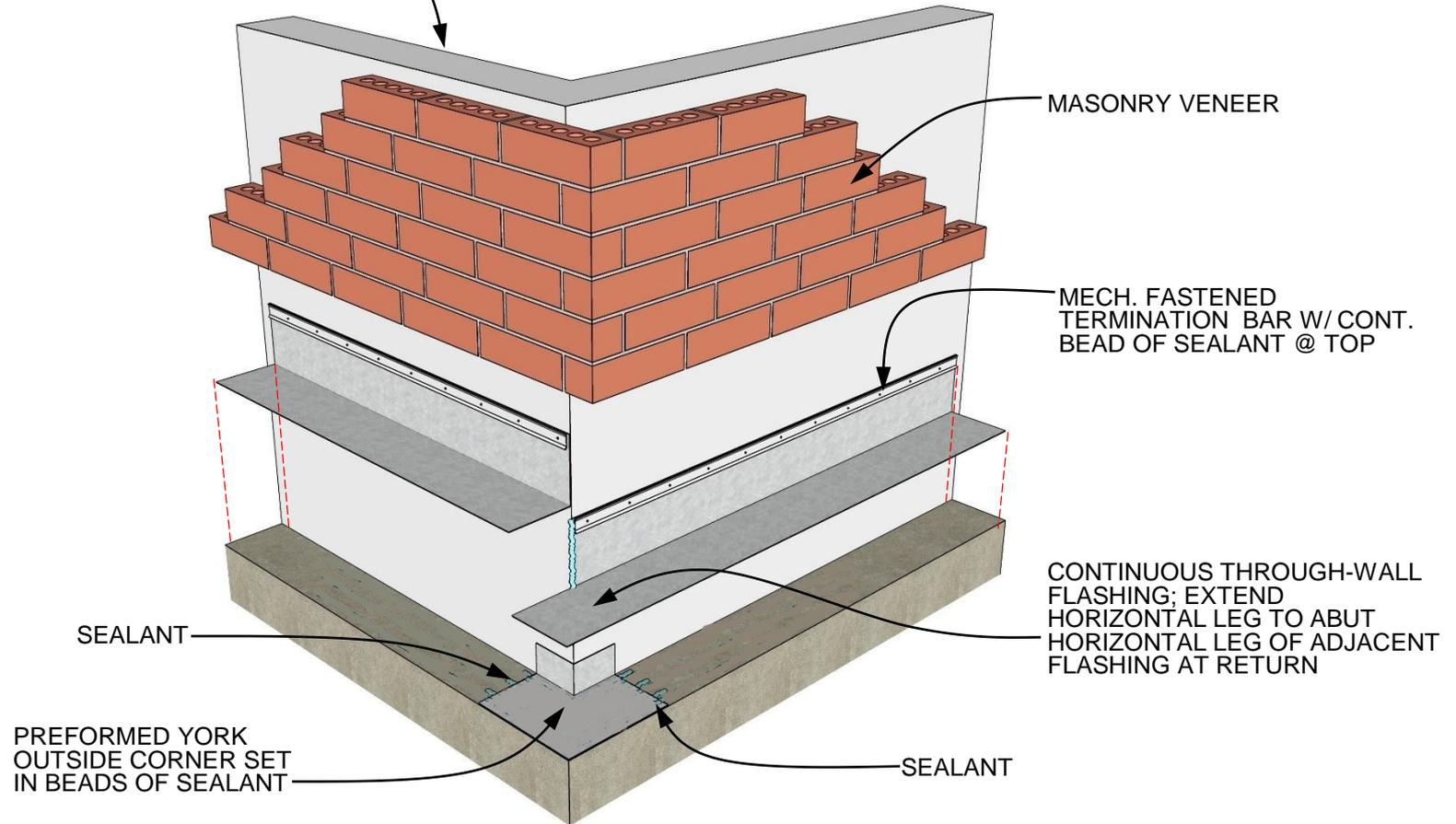
**OUTSIDE CORNER, EXPLODED VIEW YORK FLASHVENT™ MAX SELF ADHERING FLASHING**
